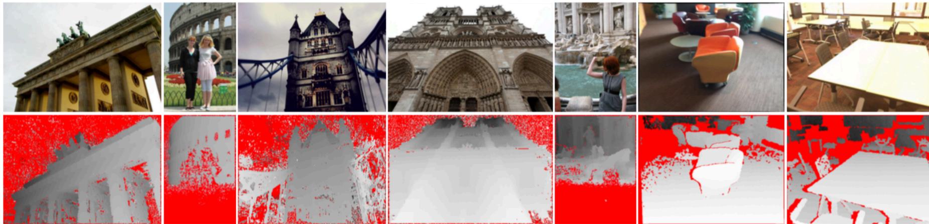
Figure 2: Samples from our indoors and outdoors datasets. Image regions without depth measurements, due to occlusions or sensor shortcomings, are drawn in red, and are simply excluded from the optimization. Note the remaining artefacts in the depth maps for outdoors images.
