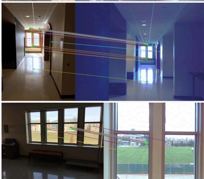
Figure 10: Examples of correctly matched image pairs from the InLoc [59] dataset. Our features are robust to significant changes in viewpoint as it can be seen in the first example. In textureless areas, our features act as an object matcher - correspondences are found between the furniture of different scenes. Sometimes, matches are even found across windows on nearby buildings.
